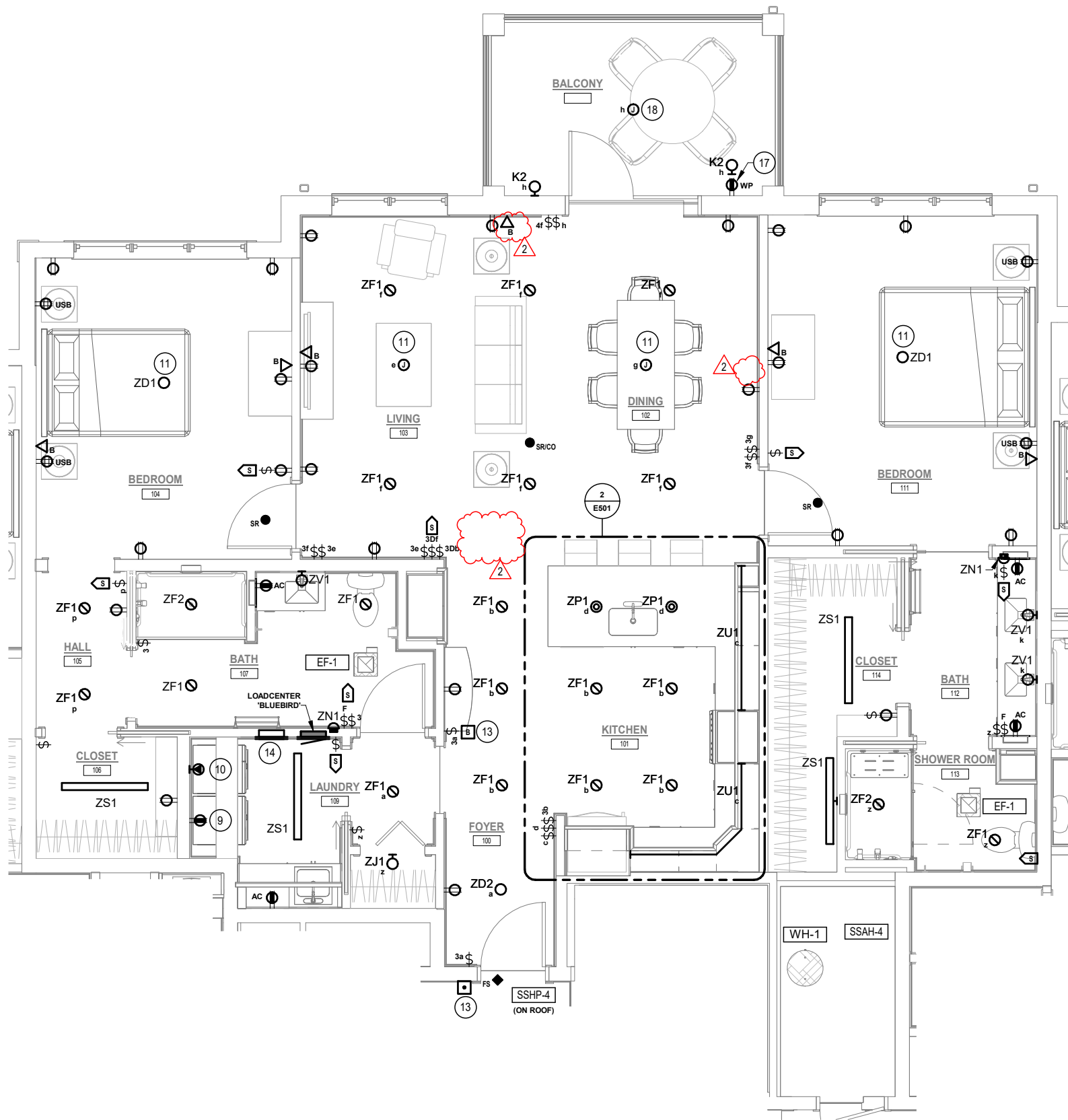
1 E501 ENLARGED 'BLUEBIRD' UNIT ELECTRICAL PLAN (ADA) SCALE: 1/4" = 1'-0"
